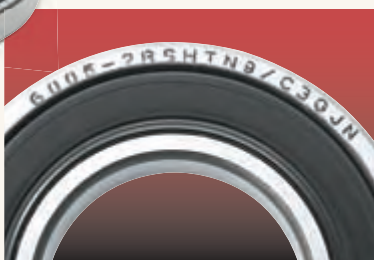
▲ New Bearings. Make sure the new bearings meet the size and speed specifications for your router.
