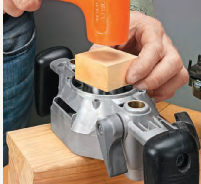
▲ Tapped In. Cut a wood block to fit over the outer race of the new bearing. When tapping it home, make sure the bearing is going in straight.
