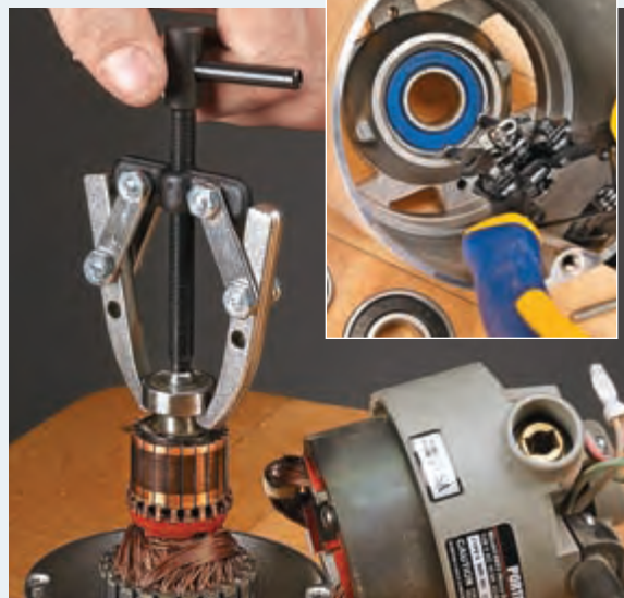
▲ Removing Bearings. Some inexpensive, but specialized tools, like a gear puller and snap ring pliers, make quick work out of removing bearings.
