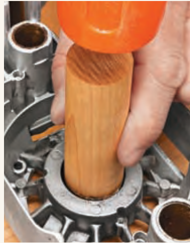
▲ Tapped Out. A dowel sized to fit the housing opening is perfect for tapping out the bearing.
