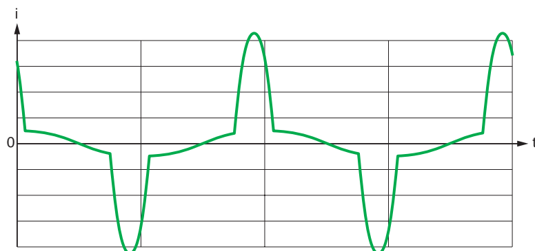
Fig. 24 : Current drawn by a load with linear and non-linear circuits
