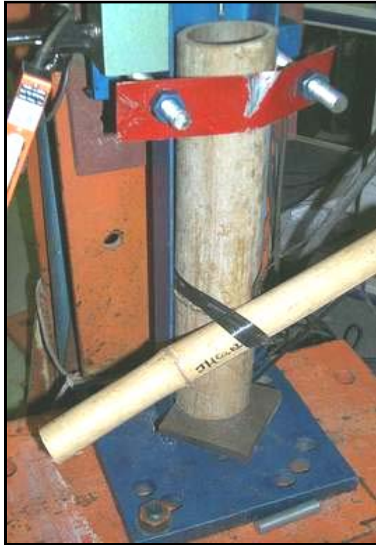
Figure 4.4 Slipping between members
