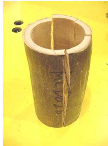
d) Typical failure mode - Splitting
