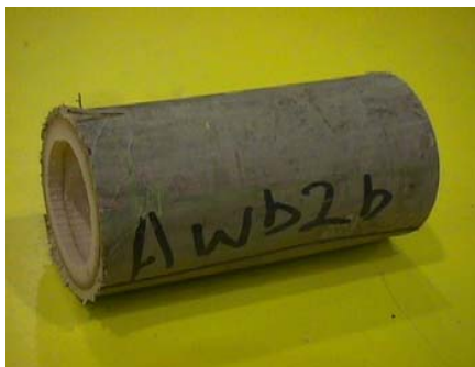
c) Typical failure mode - End bearing
