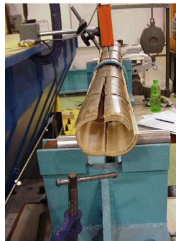
d) Typical failure mode - Splitting
