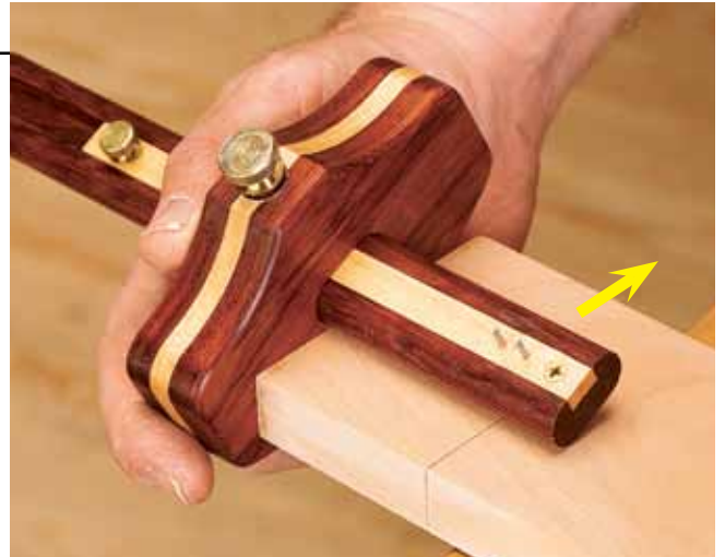
Use the single point to scribe the shoulders of a tenon...
