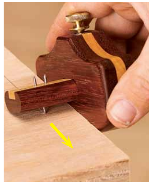
... or scribe plywood to prevent chipping when cutting rabbets.
