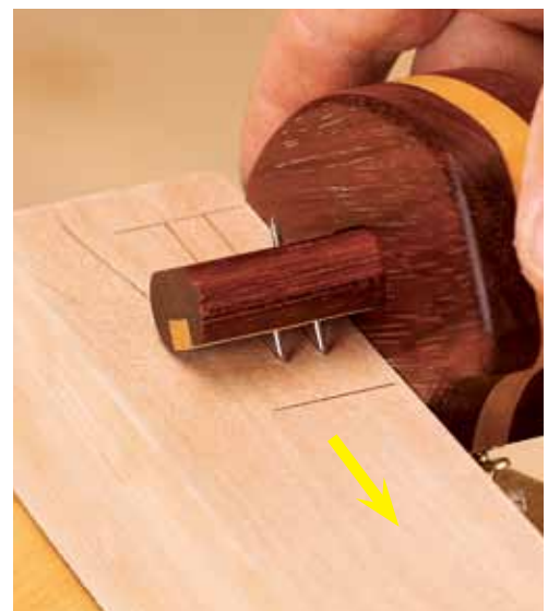
Set the paired points to the width of a tenon, and scribe mortises on your stock.
