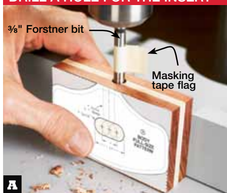
A Adhering a masking tape "flag" to a \frac{3}{8} " Forstner bit to mark the depth, drill a 1\frac{1}{8} "-deep hole centered in the body (A).
