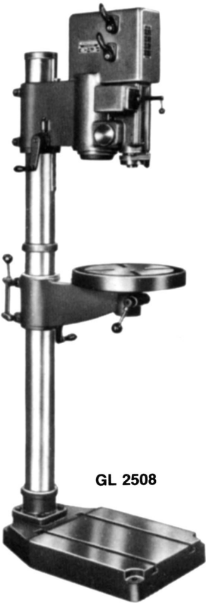
The lower spindle bearing is located as near to the gauge line as possible in order to provide the greatest degree of stability. The quill is counterpoised by means of a spring which can be adjusted to provide the ease of movement suitable for the operator. (Fig. 4.)
